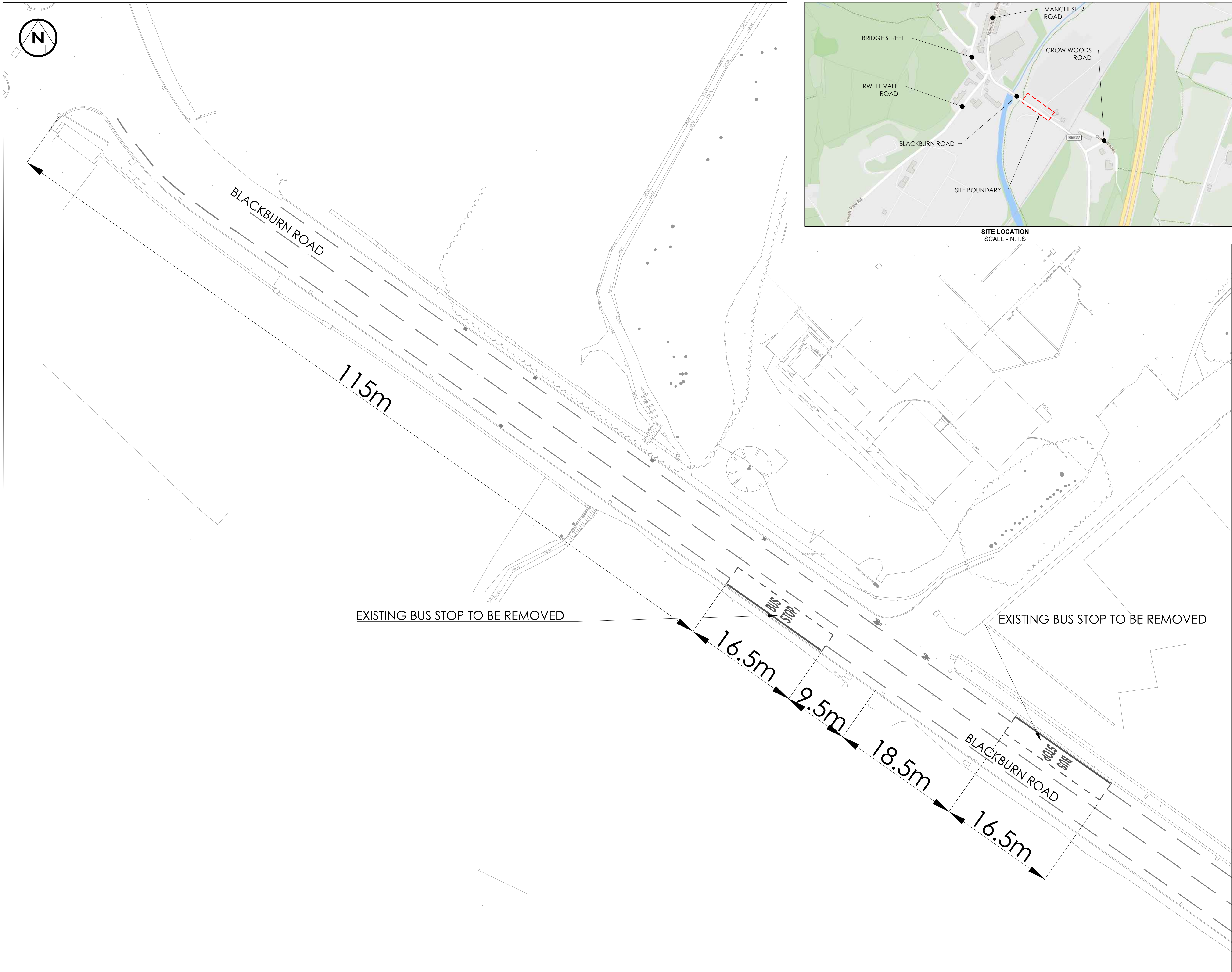
BUS STOP REMOVAL PLAN SCALE - 1:250
