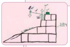
We used a lever and fulcrum. The lever was 1 metre and 6 cm long. It took 400-600 g to raise the brick up to the next level each time. The fulcrum was 1 cm each time. We used nine blocks to raise the brick up to the top of the structure so we could slide it across.
