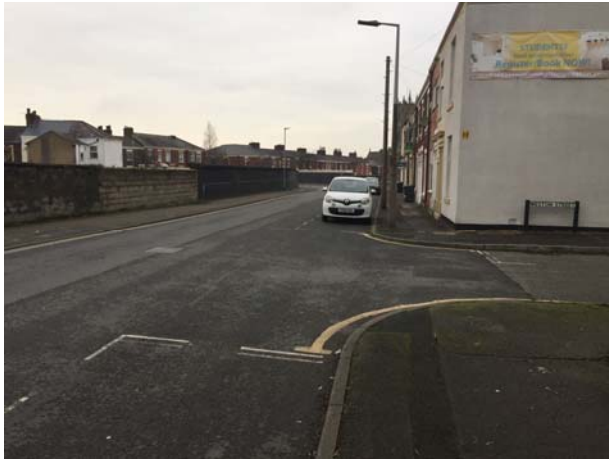
Pedder Street through to Westons – 20mph on Pedder Street and junction treatment to move parking further away from junction to improve cyclists visibility. Some localised signing improvements.
