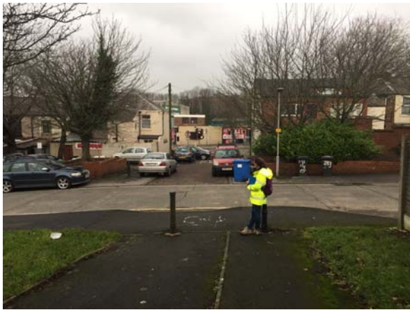
Path from Steeple view to Fylde Road – A narrowing and informal crossing of Fleetwood Street would aid route continuity. Formalising parking spaces and enforcement is needed to ensure the route through to Fylde Road isn't blocked to pedestrians / cyclists.
