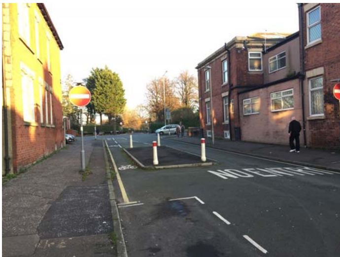
Ripon Street approach to Garstang Road junction – Cycle contra-flow lane is narrow and should be widened to help accommodate adapted cycles
