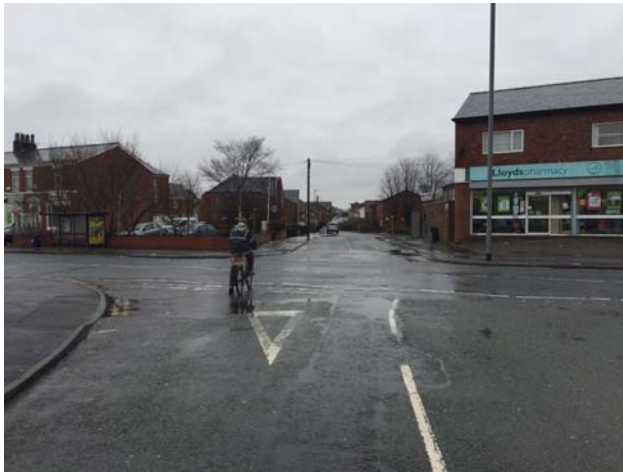
Meadow St / Deepdale Road junction – Pedestrian crossing facilities are in place but there is no provision for crossing Deepdale Road by cycle. Junction redesign is recommended to accommodate both pedestrian / cycle crossing to allow a coherent route from Meadow Street to Peel Hall Street.
