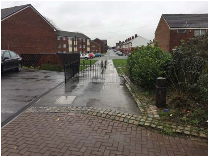
Peel Hall Street – Staggered barriers block the route making it impassable with non-standard cycles. These should be replaced with a bollard with space for mobility scooters and non-standard cycles to pass.
