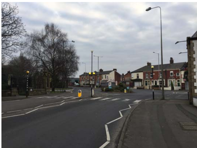
New Hall Lane / Blackpool Road roundabout – wide & fast approaches make the roundabout difficult to negotiate for pedestrians and cyclists. Recommend reducing junction radius reallocating space to pedestrians and making it easier to negotiate by cyclists.
