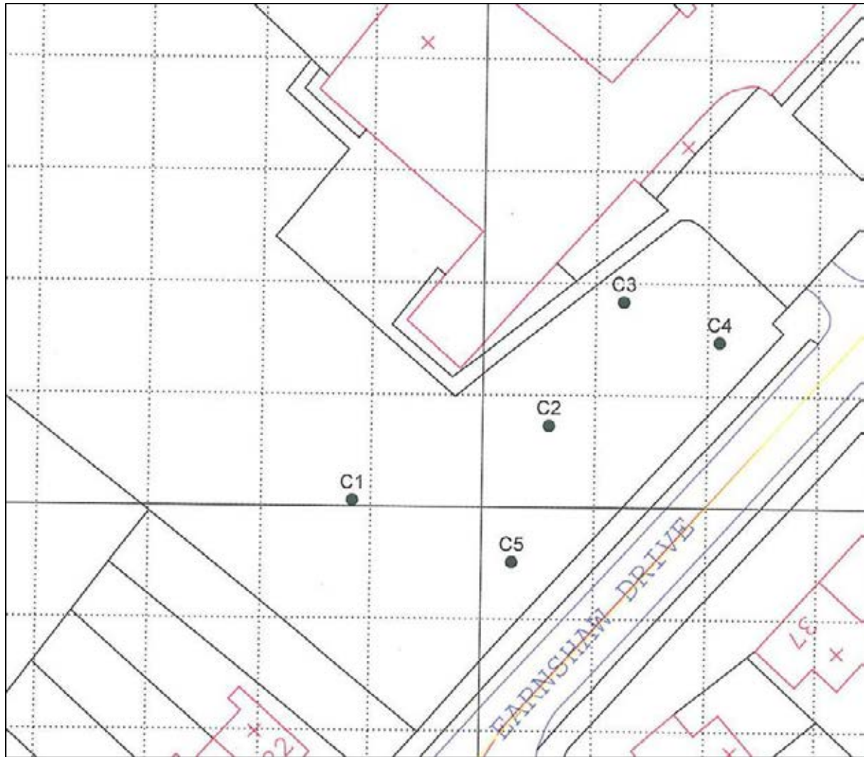
Figure 3: The borehole plan from the 2006 site investigation.
