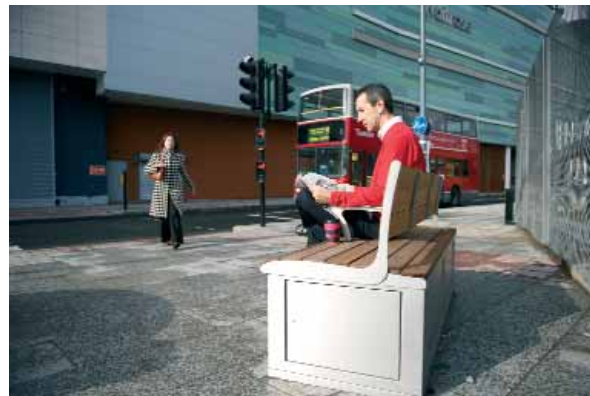
Figure 5-16 Signal control benches
